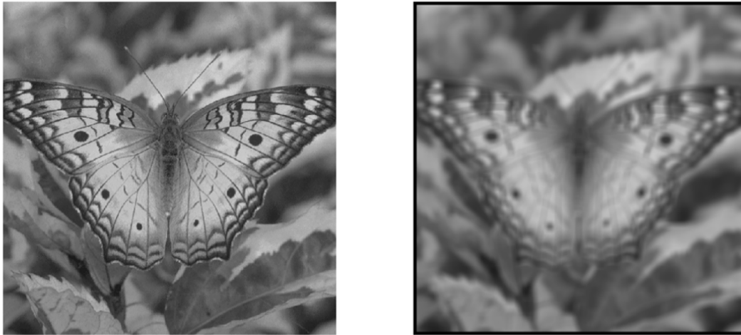
Figure 1. Two images with 512-by-512 pixels over the same area and thus the same pixel spacing. Note that the image on the right has much lower spatial resolution due to low-pass filtering.
