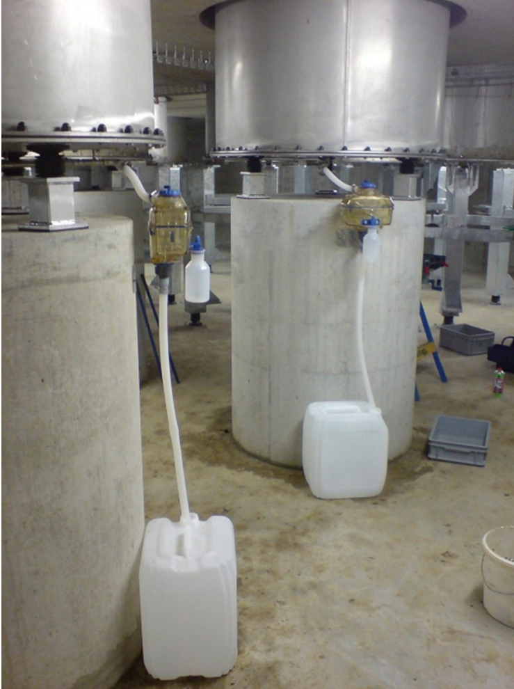
Figure A.1: Lysimeter station Reckenholz belowground (tipping buckets with sampling bottles).
