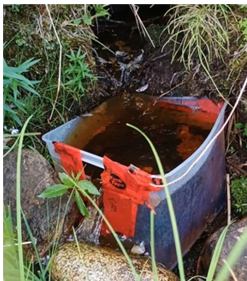
Figure A4. a) V-notch bucket weir installed at the groundwater spring in spring 2025 ~5 m from the intersection point between the transect and Tomorrow Lake, fitted with a HOBO U20L water level logger,
