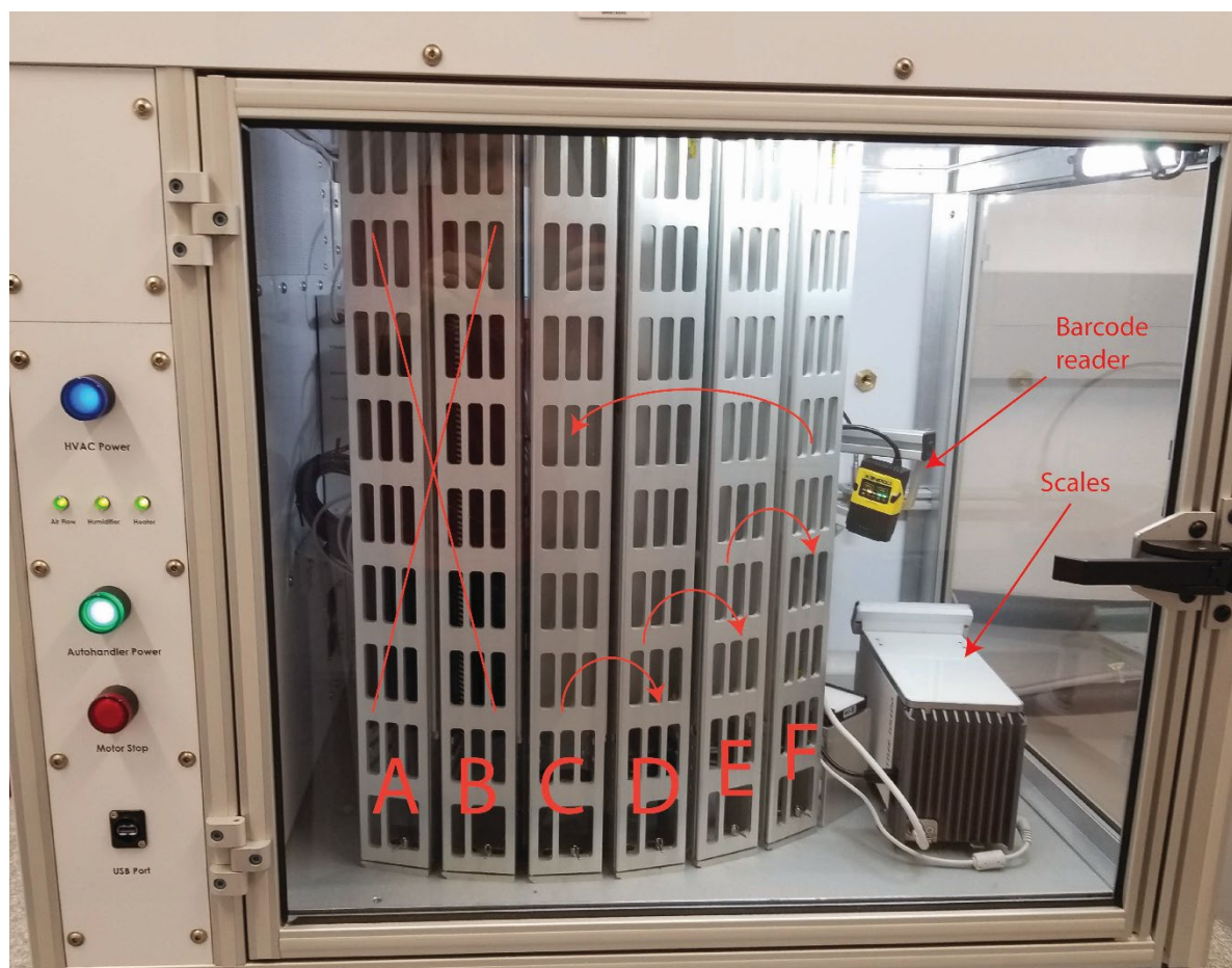
“Figure S6. The AH500 system. The silos are labeled A through F. A barcode reader is used to identify each filter. The picture shows the back side of the scales. All items behind the shown door exist inside the controlled environment described by Figure S4.
