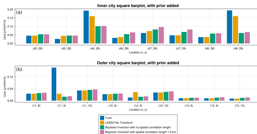
Figure G1. These barplots visualize the behavior of SR and BI in the close vicinity of point sources in the inner and outer city areas. The prior is added to the bar plots. BI smoothes over point sources and increases fluxes in the general surrounding area. SR, on the other hand, captures the location of the point source well under good conditions but can misattribute sources when they are located in the outer area, where recovery conditions are less favorable.
