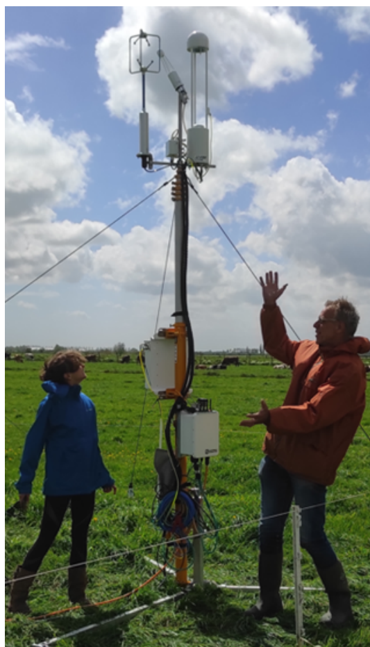
Fig. D1. Compact eddy covariance (EC) system installed in managed peat grassland. The setup includes a three-dimensional sonic anemometer and an enclosed infrared gas analyzer mounted on a stabilized mast, with data logging and power supply units.
