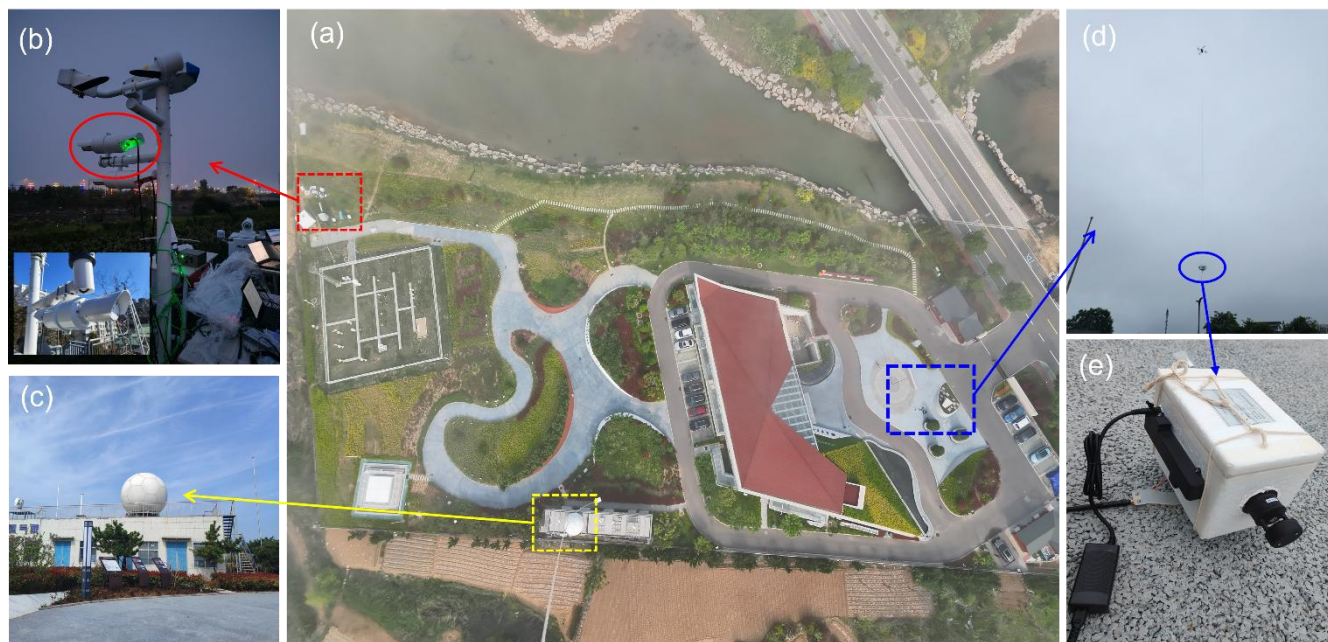
Figure 1. Experimental setup at the Huangdao observation site. (a) Aerial view; (b) ground-based droplet spectrometer and visibility sensor; (c) Ka-band cloud radar; (d) UAV during flight; (e) LCPIS probe close-up.
