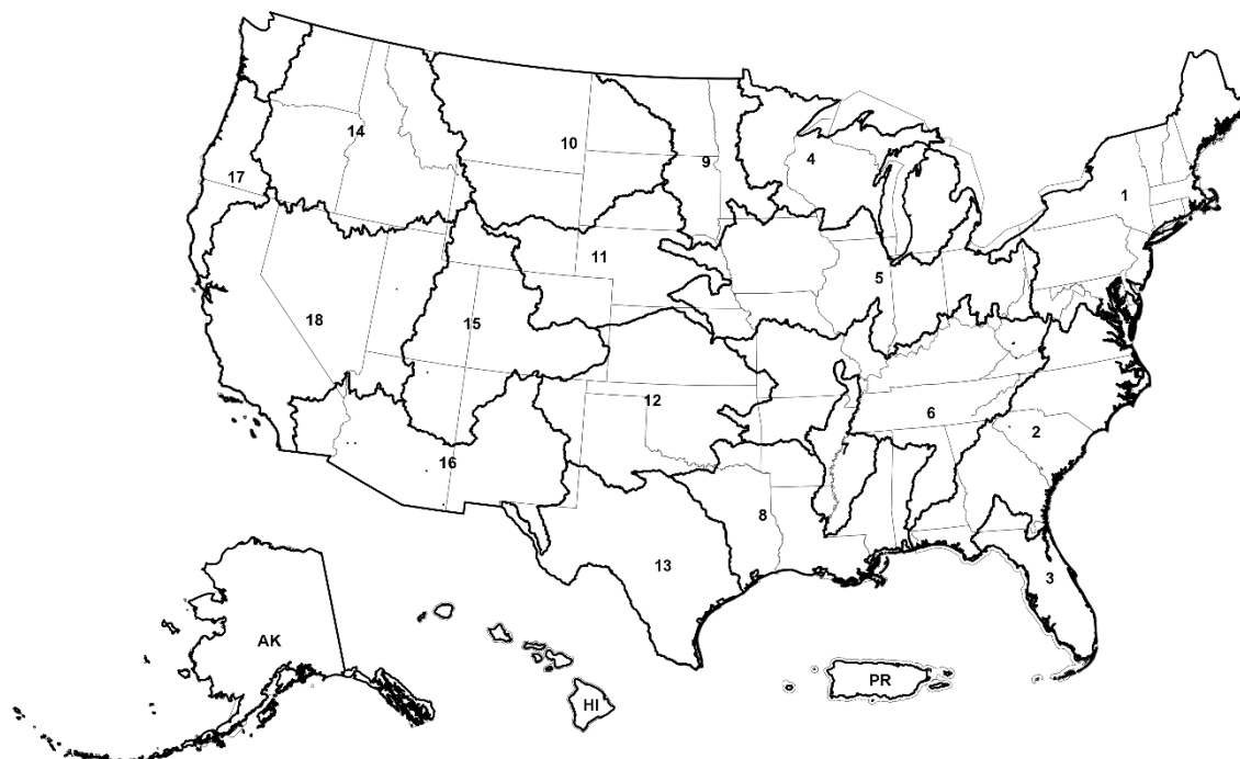
895 Figure A14: Map of CONUS, Alaska, Hawaii, and Puerto Rico with the hydrologic regions overlaid. The regions are defined as: 1 = Northeast, 2 = Atlantic Coast, 3 = Florida, 4 = Great Lakes, 5 = Midwest, 6 = Tennessee-Missouri, 7 = Mississippi Embayment, 8 = Gulf Coast, 9 = Souris-Red-Rainy, 10 = Northern High Plains, 11 = Central High Plains, 12 = Southern High Plains, 13 = Texas, 14 = Columbia-Snake, 15 = Central Rockies, 16 = Southwest Desert, 17 = Pacific Northwest, 18 = California-Nevada, AK = Alaska, HI = Hawaii, PR = Puerto Rico (Van Metre et al., 2020)
