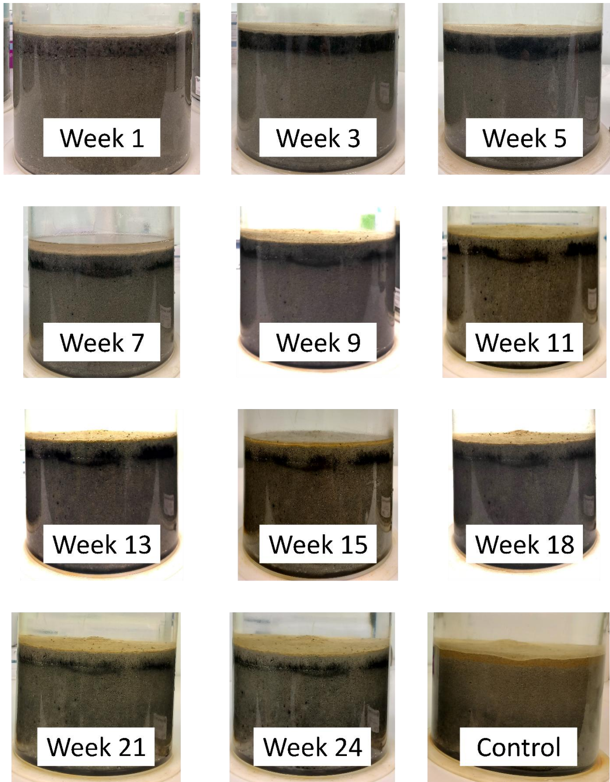
Figure S7: Pictures of shell-amended incubation chambers per week. A buildup of anoxia in the shell layer was observed, followed by the slow reoxygenation of the sediment. A picture of a control chamber, taken at the end of the experiment, was added for comparison.
