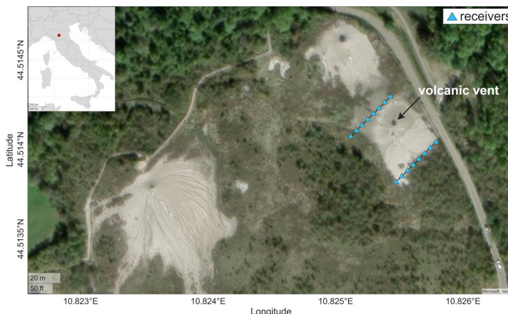
Figure 1 - Satellite image of the study area and experimental setup of the deployed seismic instruments. The blue triangles indicate the positions of the 16 vertical geophones arranged in two parallel branches with an inter-station distance of 5 m and 40 m between the two branches. The black arrow indicates the emissive point below which the array has been arranged. Background satellite imagery © Microsoft, Vantor. The map was created using ArcGIS® Pro software by Esri | Powered by Esri.
