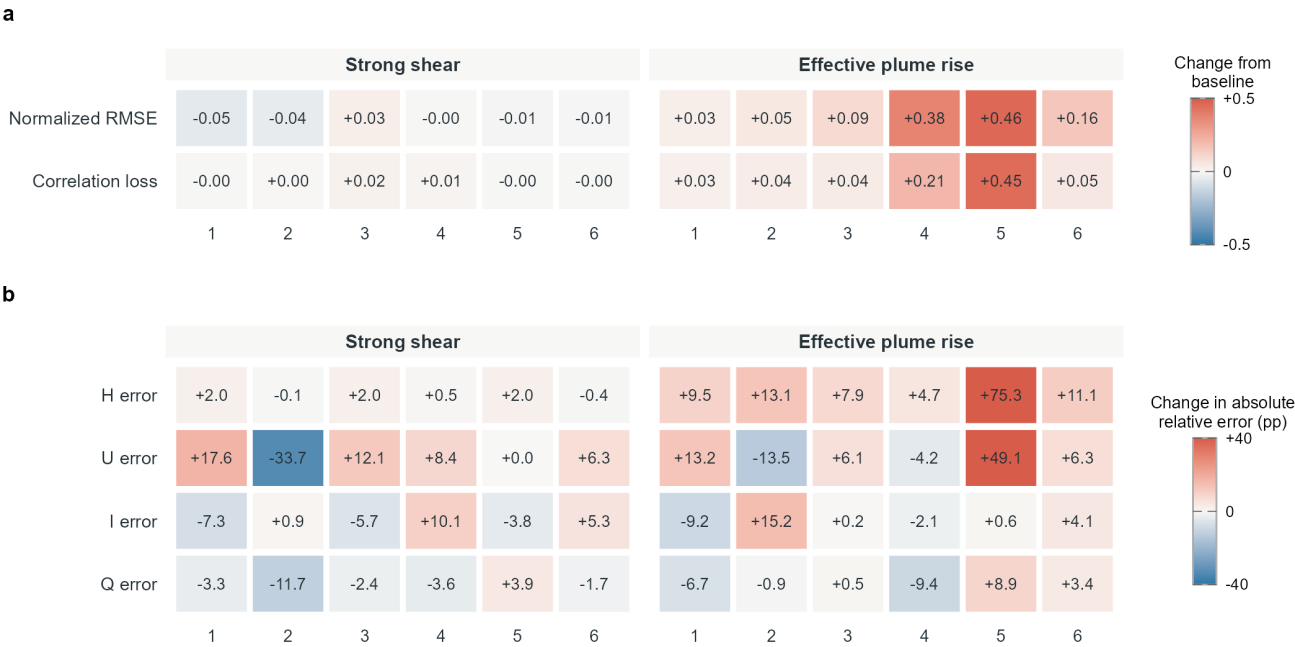
Figure F1. Controlled transport-mismatch stress tests across six representative conditions within the trained parameter support. Rows show changes in normalized RMSE, correlation loss, and the absolute relative errors of H , U , I , and Q ; columns identify Cases 1–6 for each mismatch condition. Changes are relative to each case’s simple-transport baseline under the same 1% random-volume observation mask. Positive values denote worse performance, with correlation loss defined as baseline minus tested spatial correlation. Cell labels report un-truncated changes; parameter-error colors are truncated at \pm 40 percentage points to preserve contrast.
