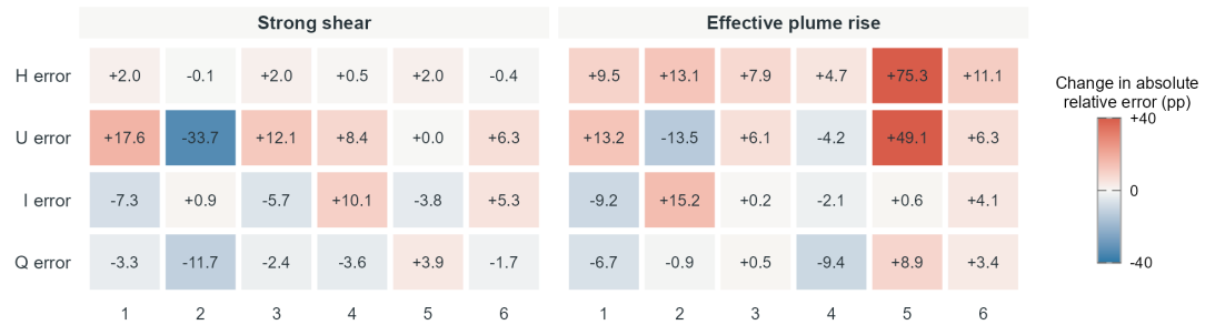
Appendix Fig. F1. Controlled transport-mismatch stress tests across six representative conditions within the trained parameter support. Rows show changes in normalized RMSE, correlation loss, and the absolute relative errors of H , U , I , and Q ; columns identify Cases 1--6 for each mismatch condition. Changes are relative to each case's simple-transport baseline under the same 1% random-volume observation mask. Positive values denote worse performance, with correlation loss defined as baseline minus tested spatial correlation. Cell labels report untruncated changes; parameter-error colors are truncated at \pm 40 percentage points to preserve contrast.
