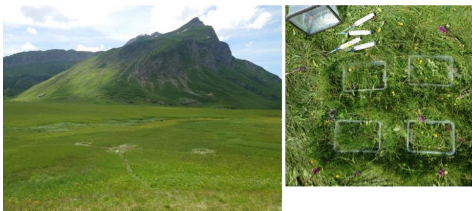
Fig. A3. Pictures of the group-wise setup of the chambers within the Auenfeld alpine peatland. Left: overview with the three groups visible. Right: the setup of the 4 chambers within one group.
