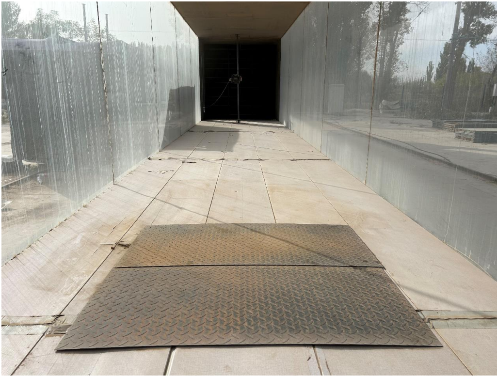
Photograph of the test section after the original soil source bed was covered with steel plates. The plates remained in place throughout the low-wind accumulation phase.
