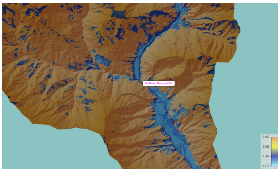
Figure 4: Spatial distribution of Manning’s roughness coefficients ( n ) derived from LULC and soil data.
