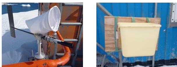
140 Figure 2: Manual snow collection setup. Left: sock mounted on a wind vane, designed to collect blowing snow. Right: open tray, preferentially capturing vertically falling snow.
