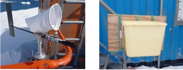
180 Figure 2: Manual snow collection setup (1 m above ground level). Left: sock mounted on a wind vane, designed to collect blowing snow. Right: open tray, preferentially capturing vertically falling snow.
