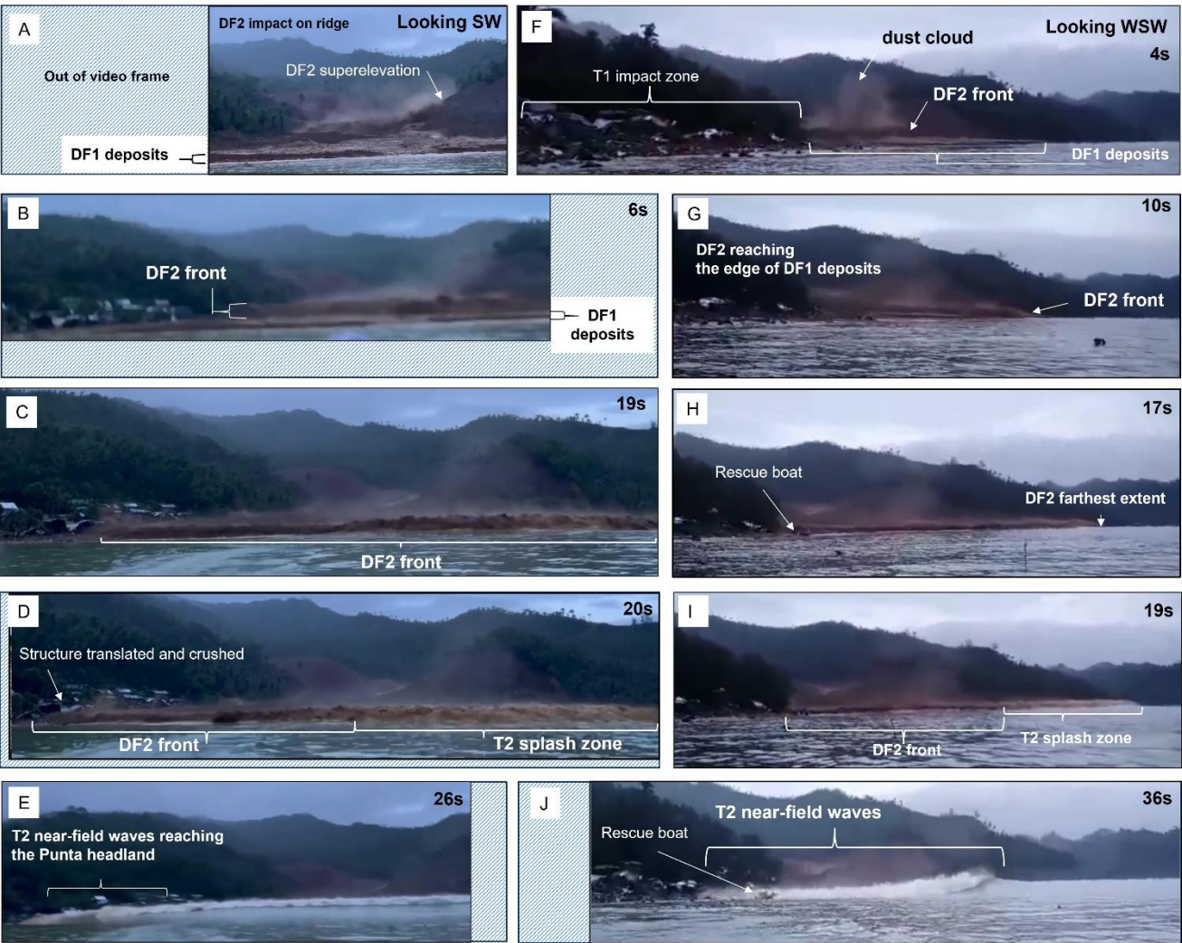
Figure 7: Frames from videos taken by rescuers at Pilar as DF2 flowed over DF1, reached the shore and generated Tsunami 2 (T2) (A-E: looking southwest c/o PDRRMO, 2022; F-J: looking west-southwest c/o BFP Region VIII, 2022).
