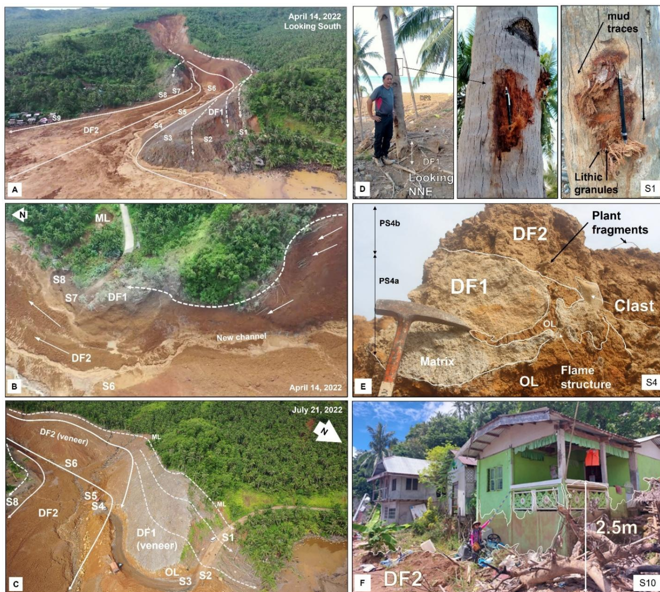
Figure 6: Debris flow directions based on the orientation of toppled trees and depositional structures (DF1 dashed; DF2 solid arrows). A) April 14, 2022 drone footage posted by GPM TV Philippines via Youtube. Field survey stations in July 2022 are marked (S1 to S9). B) New channel formed after DF1 & DF2. C) Superlevation marks on the western extent of DF1 & DF2 on a ridge underlain by an older landslide deposit (OL). D) The runup height (1.8m) of DF1 as indicated by scratches on coconut trees along the main road at S1. E) The contact between OL, DF1 and DF2 along the new roadcut, where soft-sediment deformation (flame structure) was observed at the contact of DF1 with OL at S4. F) House at S10, along the edge of DF2 deposits where debris flow runup of 2.5m was observed.
