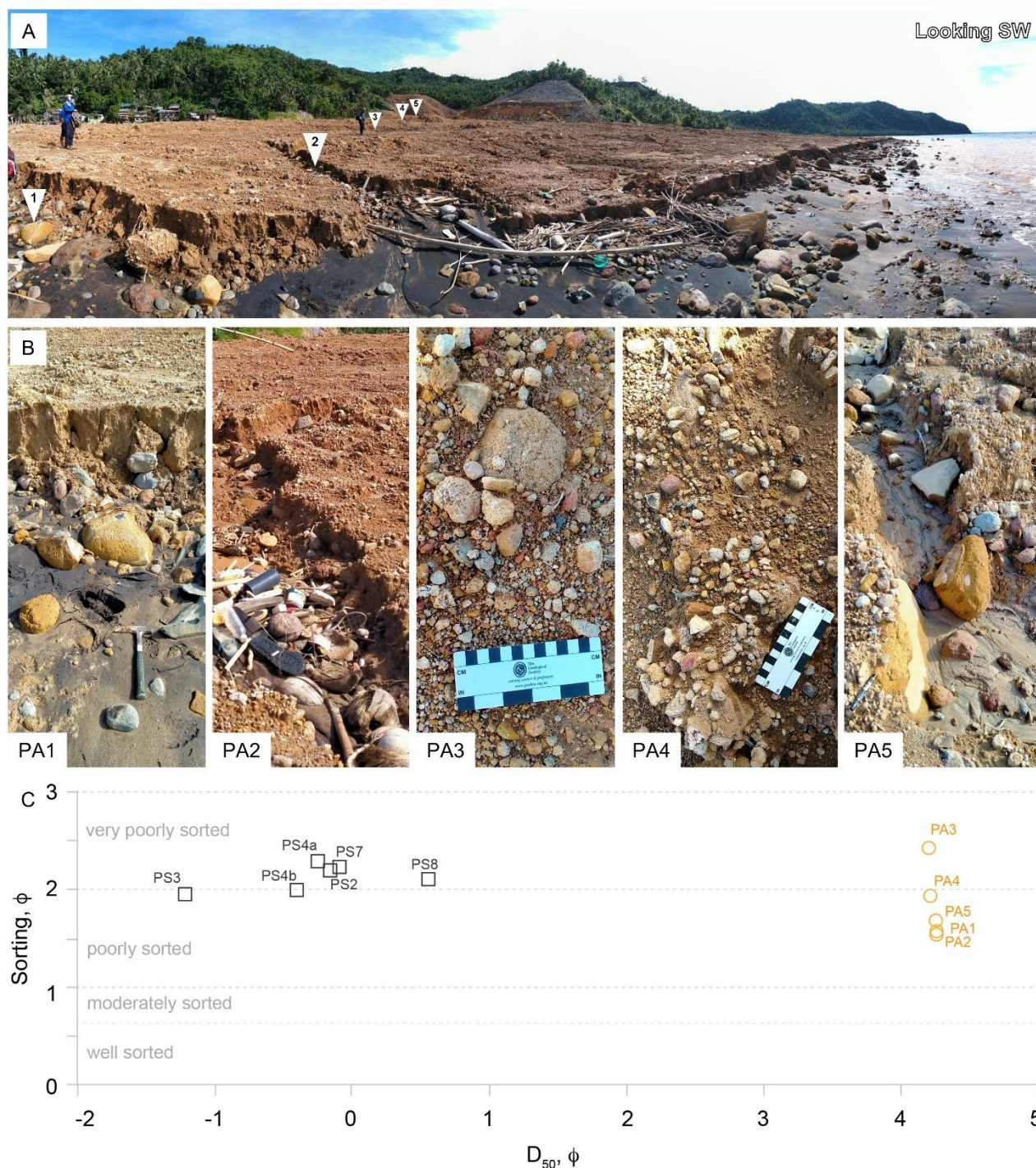
Figure 8: Auger Sampling Stations (A1 to A5). A) Panoramic shot at the July 19, 2022 coast of Pilar; inverted triangles marking the Auger Sampling points. B) Surface of DF2 sample sites. C) Sediment Analysis of DF1 (gray squares) and DF2 (brown circles) samples.
