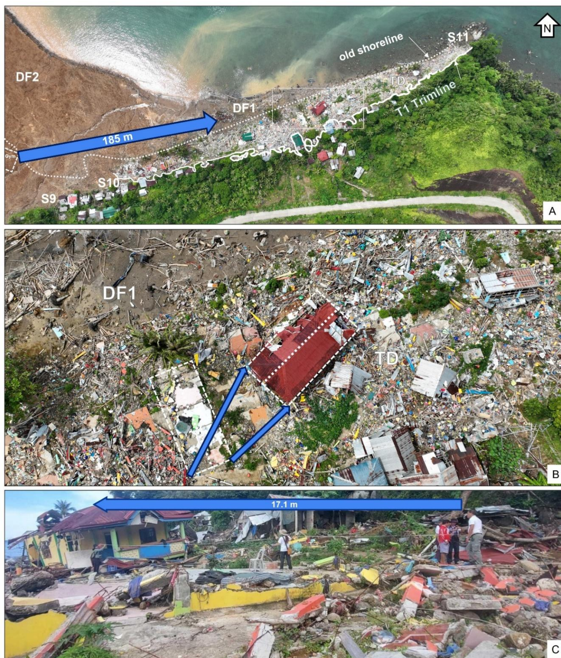
Figure 10: Landslide-Tsunami impact in Pilar. A) Extent of the tsunami impact zone. The white rectangle marks the extent of the next photo. Blue arrow shows the displacement of the Barangay gym. B) UAV photo of the tsunami debris (TD) field. The dashed white rectangles outline the red-roofed house and its foundation. Blue arrow indicate the displacement direction of its southern corners. C) Destruction and displacement of structures caused by the tsunami (T1) as seen from the ground.
