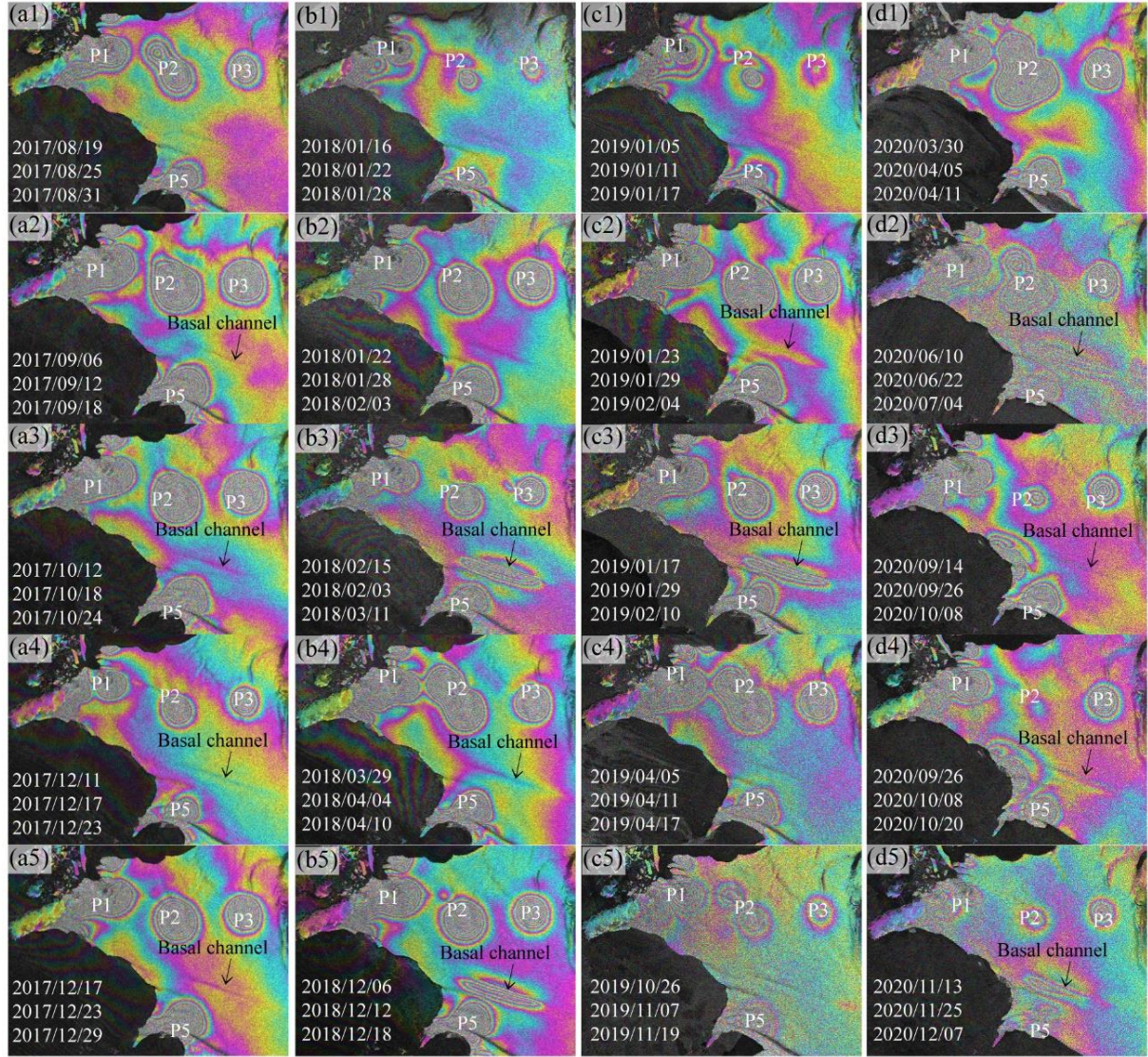
Figure 8. Changes in pinning points P1, P2, P3, and P5 derived from double-difference interferograms over the N-PIIS from 2017 to 2020. Panels (a–d) show results for 2017, 2018, 2019, and 2020, respectively.
