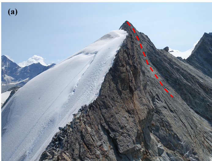
Figure S4: (a) Main summit of PdM, view of the hanging glacier on its north face, and the west face with 120 m long ERT 1 profile, SW branch, marked in red. (b) Profile ERT 1, SW branch, view from PdM summit.
