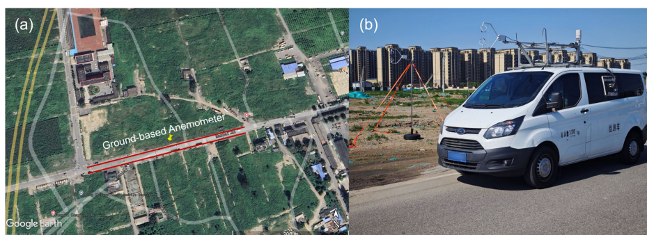
Figure 5: Field validation site and deployment of the ground-based anemometer. (a) Satellite image of the validation site, where the yellow marker indicates the location of the ground-based anemometer and the red lines denote the vehicle driving trajectories
