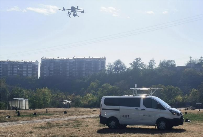
Figure S1: Vehicle geometry reconstruction based on UAV-mounted LiDAR measurements.
