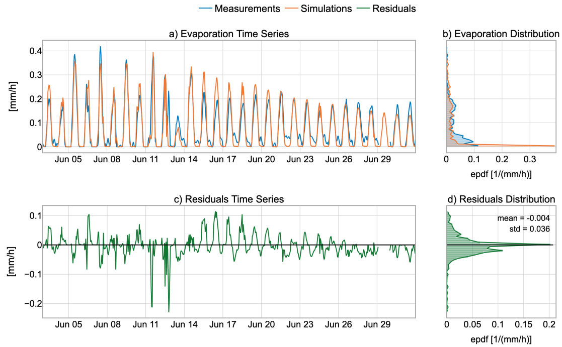
Figure S4: Multidimensional analysis of evaporation time series and distributions in L3 lysimeter simulation: A comparison between evaporation measurements and simulations. Panels a) and b) depict time series and distributions of evaporation, while Panels c) and d) highlight residuals and their distributions.
