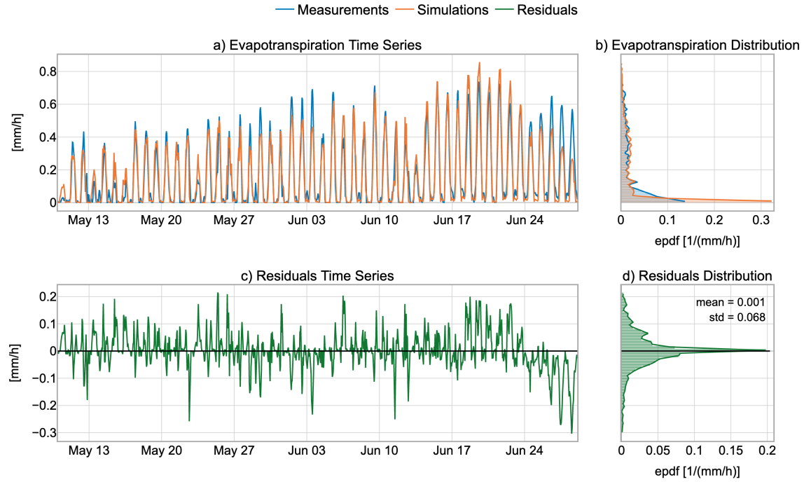
Figure S2: Multidimensional analysis of evapotranspiration time series and distributions in L1 lysimeter simulation: A comparison between evapotranspiration measurements and simulations. Panels a) and b) depict time series and distributions of evapotranspiration, while Panels c) and d) highlight residuals and their distributions.
