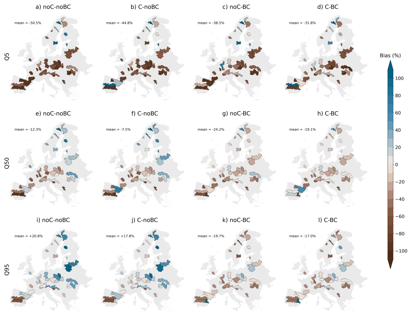
Figure 5. Percentage bias at low (Q05, upper row), median (Q50, middle row), and high (Q95, bottom row) flow levels of C-CWatM model simulations from 1999 to 2008 compared to observed discharges from 40 gauging stations. Percentage biases are shown for each basin under four scenarios. (1st column) noC-noBC: no calibration and no bias-correction, (2nd column) C-noBC: calibration and no bias-correction, (3rd column) noC-BC: no calibration and bias-correction, and (4th column) C-BC: calibration and bias-correction.
