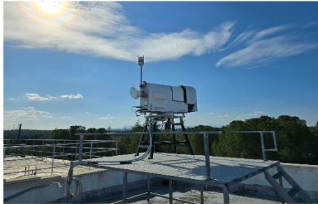
105 Figure 1. Location and instrumentation at Athalassa, Cyprus. (a) Site location on the island's elevation map. (b) GNSS reference station. 106 (c) RPG-HATPRO radiometer. (d) Radiosonde balloon launching. 107
