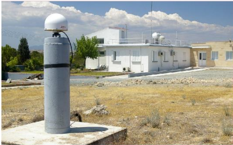
105 Figure 1. Location and instrumentation at Athalassa, Cyprus. (a) Site location on the island's elevation map. (b) GNSS reference station. 106 (c) RPG-HATPRO radiometer. (d) Radiosonde balloon launching. 107
