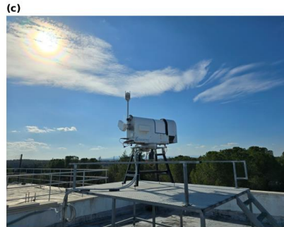
Figure 1. Location and instrumentation at Athalassa, Cyprus. (a) Site location on the island's elevation map. (b) GNSS reference station. (c) RPG-HATPRO radiometer. (d) Radiosonde balloon launching.
