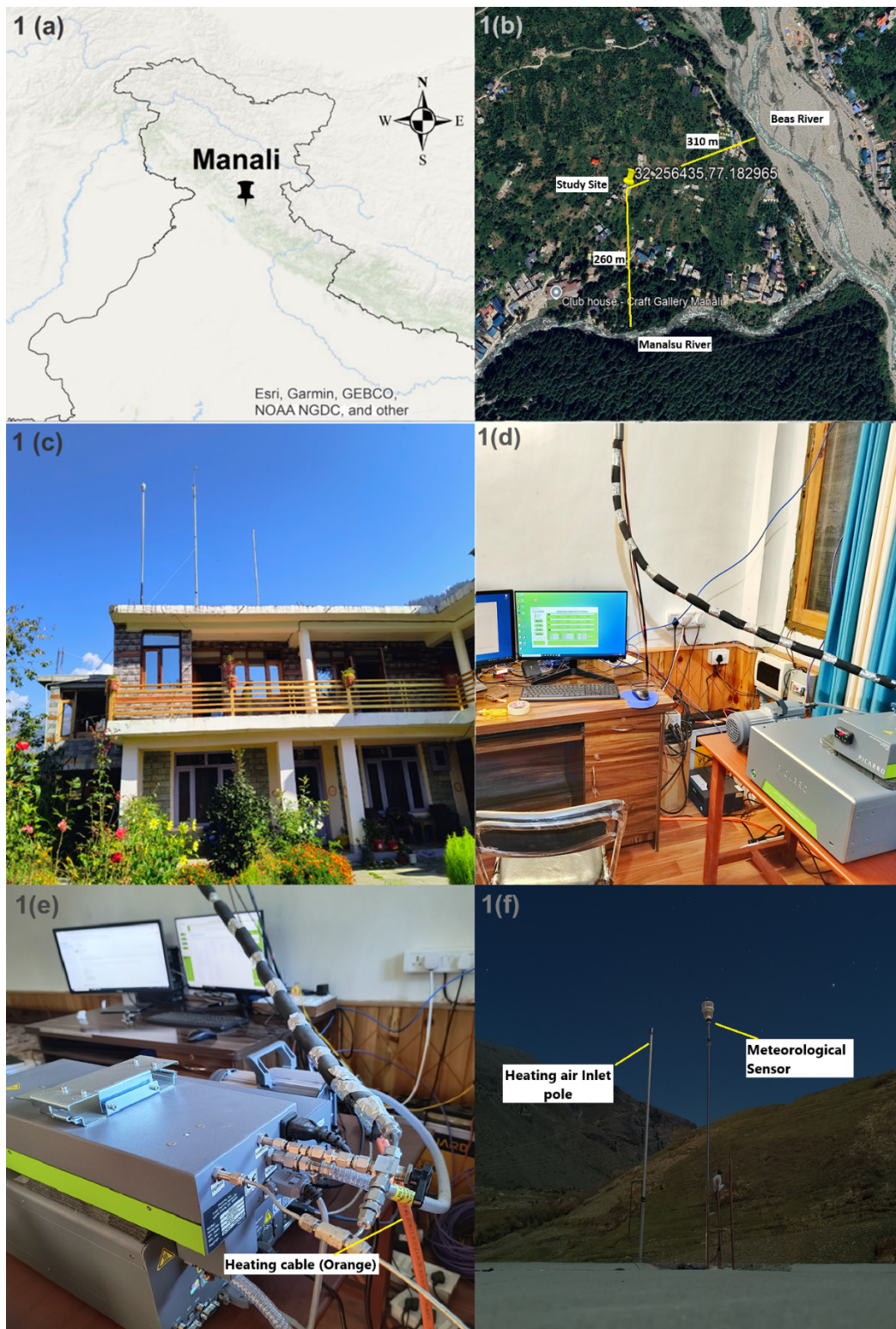
Figure 1: The heated inlet line (visible in orange/insulated jacket Figure 1(e)) is continuing without interruption from the roof penetration to the vaporizer inlet port. And Sissu deployment site Figure 1 (f) where the instrument runs for five days is located on the leeward side.
