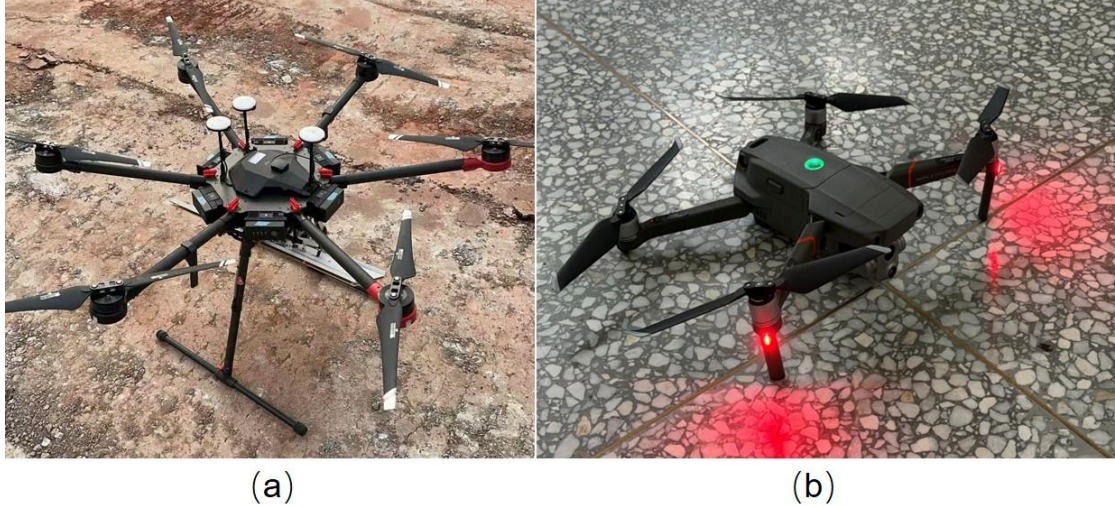
Figure 1. Field deployment of the UAV sensing system, including the (a) DJI Matrice 600 platform carrying the PoLRa v3.1 dual-polarized L-band radiometer and the (b) DJI Mavic 2 Enterprise Advanced used for RGB-TIR survey.
