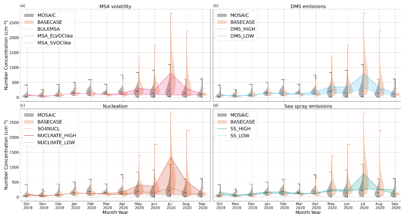
Fig. 3: Violin plot of the daily average CN from the MOSAiC expedition and the simulation, BASECASE, along the MOSAiC track. MOSAiC and BASECASE values are plotted as the left and right half violin, respectively, with the shaded area showing the probability density function of the CN values. The horizontal lines at the top and bottom of the violins represent the maximum and minimum, and the line in the middle is the median. The four subplots show the sensitivity of the model to perturbing parameters related to MSA volatility (a), DMS emissions (b), Nucleation (c) and Sea Spray emissions (d), with the lines showing the median values of the experiment and the shaded region showing the difference between the lowest and highest values.
