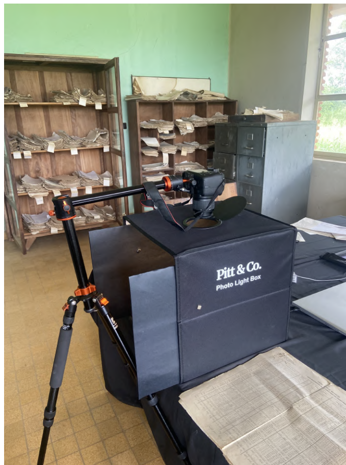
Figure 5. Digitization campaign setup at the INERA-Section de Climatologie archives in Yangambi, including a digital camera mounted on a tripod and a photobox equipped with lighting fixtures to ensure high-quality digital copies of the historical weather records. Photograph taken on 15 August 2023.
