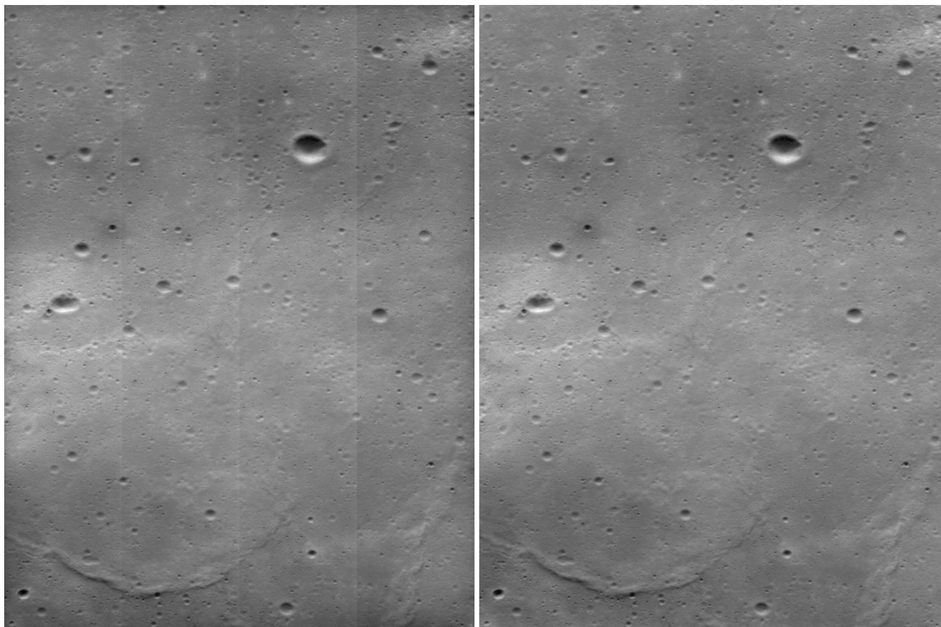
Figure 6. Partially (left) and fully calibrated (right) version of the same image. The vertical striping, introduced by the readout electronics, are removed after the absolute radiometric correction module
