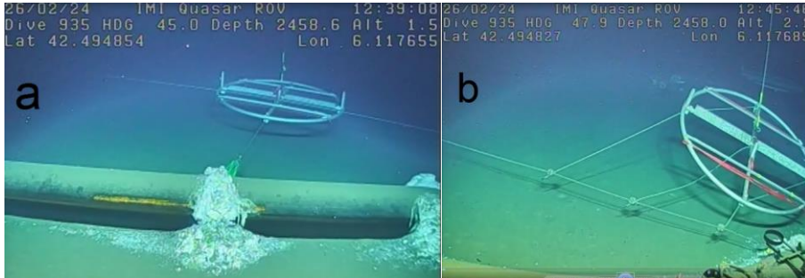
454 455 Figure 2. Underwater video stills of small-rings demonstrating steel-cable grid elevation and cable- 456 inclinations. The 0.61-m diameter steel pipe in the foreground is part of the large anchoring ring, which 457 sank 0.07 \pm 0.02 m in the sediment of the < 1^\circ flat seafloor. All steel cables are attached to the middle of 458 the steel pipes, and thus at height h = 0.24 m above sediment. (a) Line 44 (cf. Fig. 1c). To the right of 459 the small-ring the wire visibly makes a larger angle to the horizontal than to the left. (b) Estimating 460 height of ‘corner-line’ 47, see text. (Images from video by ROV Holland I). 461
