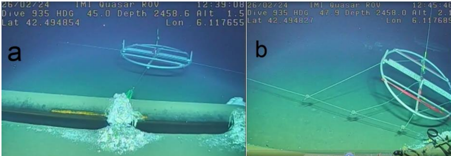
466 467 Figure 2. Underwater video stills of small-rings demonstrating steel-cable grid elevation and cable- 468 inclinations. The 0.61-m diameter steel pipe in the foreground is part of the large anchoring ring, which 469 sank 0.07 \pm 0.02 m in the sediment of the < 1^\circ flat seafloor. All steel cables are attached to the middle of 470 the steel pipes, and thus at height h = 0.24 m above sediment. (a) Line 44 (cf. Fig. 1 cb ). To the right of 471 the small-ring the wire visibly makes a larger angle to the horizontal vertical than to the left. (b) Estimating 472 height of ‘corner-line’ 47, see text. (Images from video by ROV Holland I).
