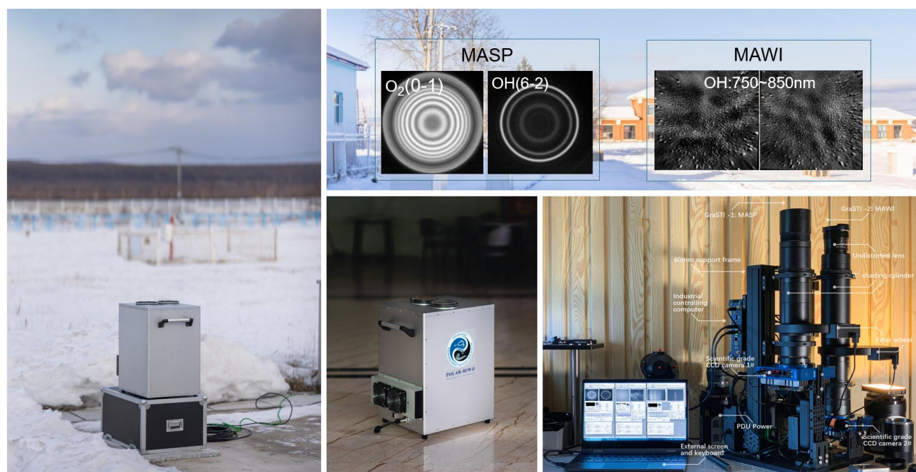
Figure 1: Photograph of the observation setup at Tulihe, together with representative MASP dual-channel airglow images in the O 2 100 (0-1) and OH (6-2) bands and a representative from MAWI.
