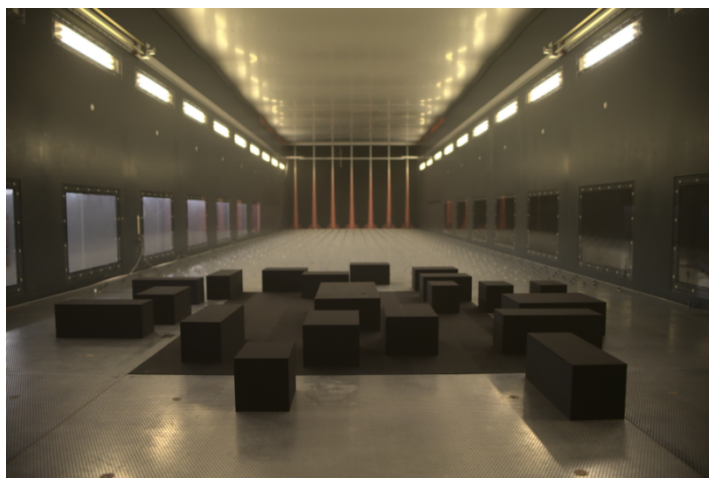
Figure 2: Idealized industrial park model inside the WOTAN wind tunnel. View from the rear of the wind tunnel looking toward the model along the x-axis. (form Michel, 2023)
