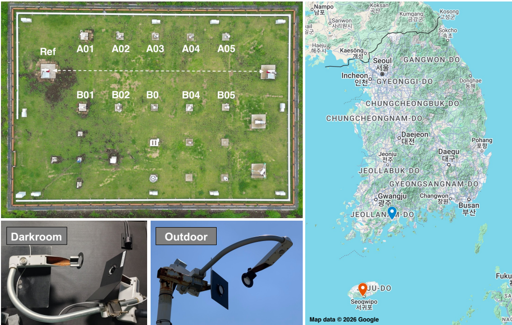
205 Figure 4: Experimental setting and site context of the present study. Top left: aerial view of the NIMS outdoor visibility-instrument test site at Seogwipo, Jeju Island, South Korea, showing the reference transmissometer (“Ref”) and the forward-scatter sensor positions used in the broader observation array. Right: map of South Korea showing the locations of the NIMS headquarters and test site at Seogwipo (orange marker) and the Boseong standard observation site (blue marker), both operated by the National Institute of Meteorological Sciences (NIMS), Korea Meteorological Administration (KMA). Map data © 2026 Google. Bottom left: 210 indoor darkroom configuration of a forward-scatter sensor equipped with the multi-filter mount used for controlled calibration measurements. Bottom centre: outdoor configuration of the same multi-filter mounting concept used during field filter tests.
