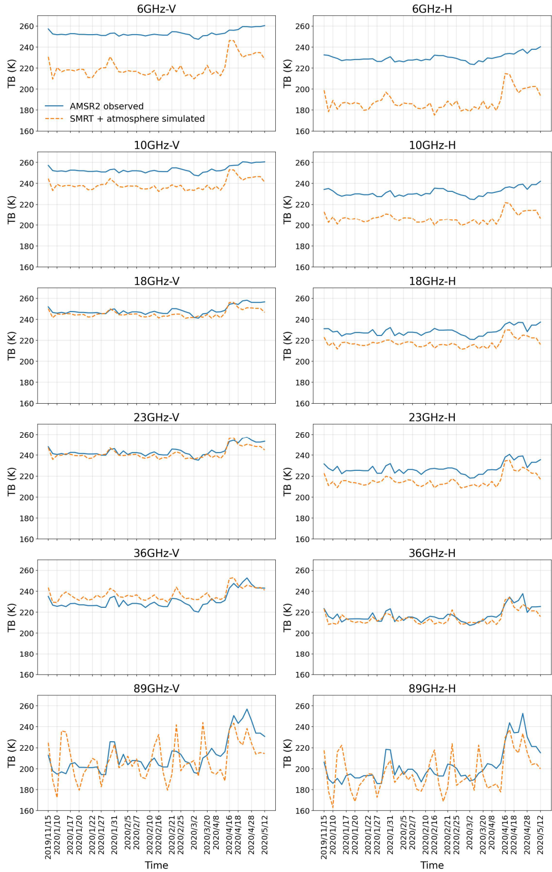
Fig. R2 Time-series comparison of SMRT-simulated TBs and AMSR2-observed TBs during the MOSAiC winter period.
