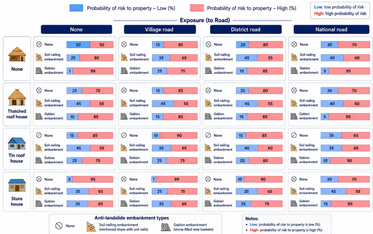
Figure 9. Probability of risk to building and road under the protection of different anti-landslide embankment.
