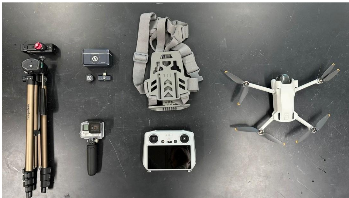
Figure 8. One lesson learned during the Collectors Tour is the reality that filming adds to the load that needs to be carried to each field site. This photo presents an overview of the additional equipment that was carried, including a camera tripod (left) a wireless microphone (upper left), GoPro camera (lower left), a chest harness for the drone controller (centre top), the drone controller (centre bottom), and a DJI Mini 3 Pro drone (right).
