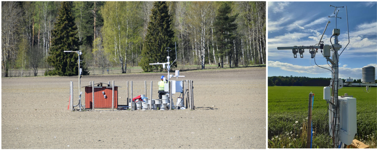
Figure 1: Left: Field installation of the reference (left tower) and the prototype (right tower) eddy covariance systems at Haltiala test site. Right: The prototype setup with Metek uSonic-3 anemometer.
