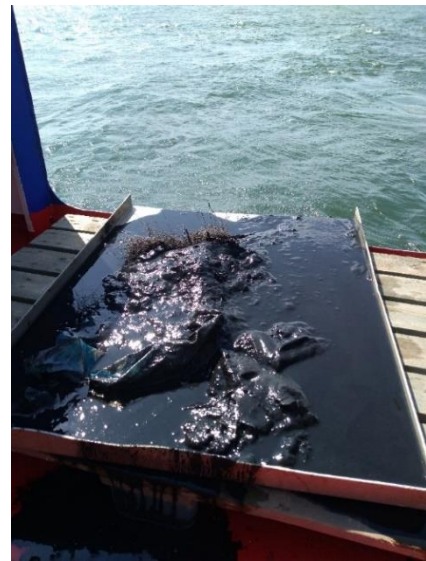
Image of mud from MET1-BH pockmark sampled with Van Veen grab (Foto: Olga Broclawik)
