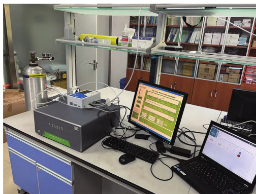
Figure S2: Demonstration of the testing procedures using the LICOR-830 and Picarro G2301
