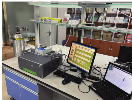
Figure R-1: Demonstration of the testing procedures using the LICOR-830 and Picarro G2301 instruments in the laboratory
