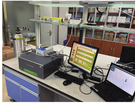
Figure R-1: Demonstration of the testing procedures using the LICOR-830 and Picarro G2301 instruments in the laboratory
