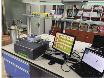
Figure S-1: Demonstration of the testing procedures using the LICOR-830 and Picarro G2301 instruments in the laboratory
