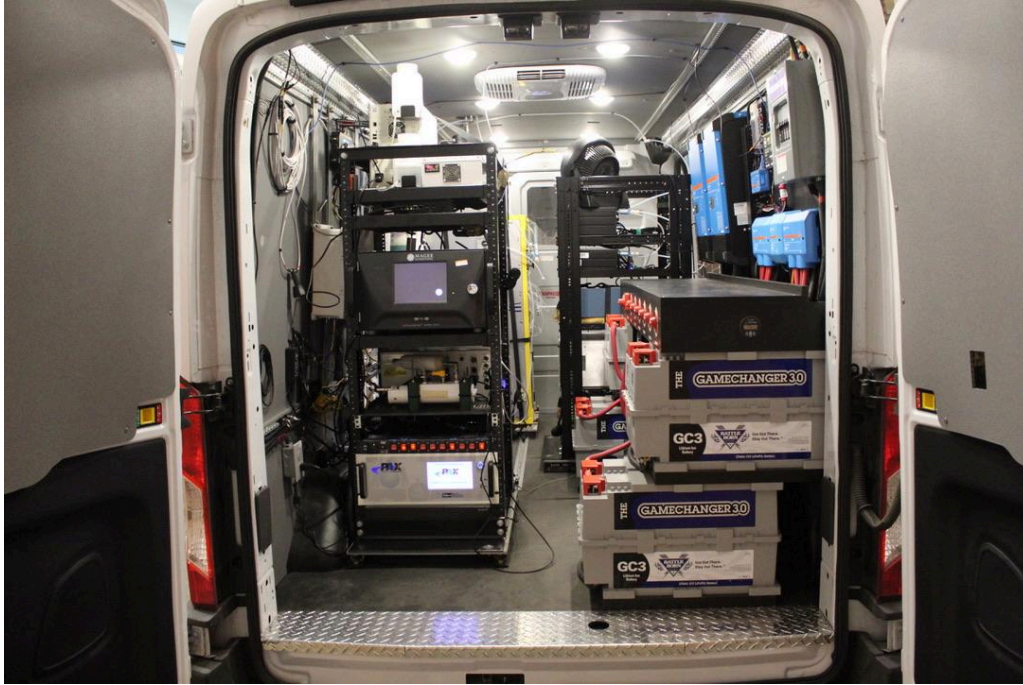
Figure S2: View of the CalMAPLab through the rear cargo doors. On the left is the mostly particle phase rack containing the TSI CPC, Magee AE33, Spider Magic, Palas Fidas, DMT PAX and the Licor CO 2 instruments. It also hosts the van server wired into the router and rooftop antennae through the white cables. On the right is the battery electric system with batteries on the bottom and inverters, busbars and fuse boxes above.
