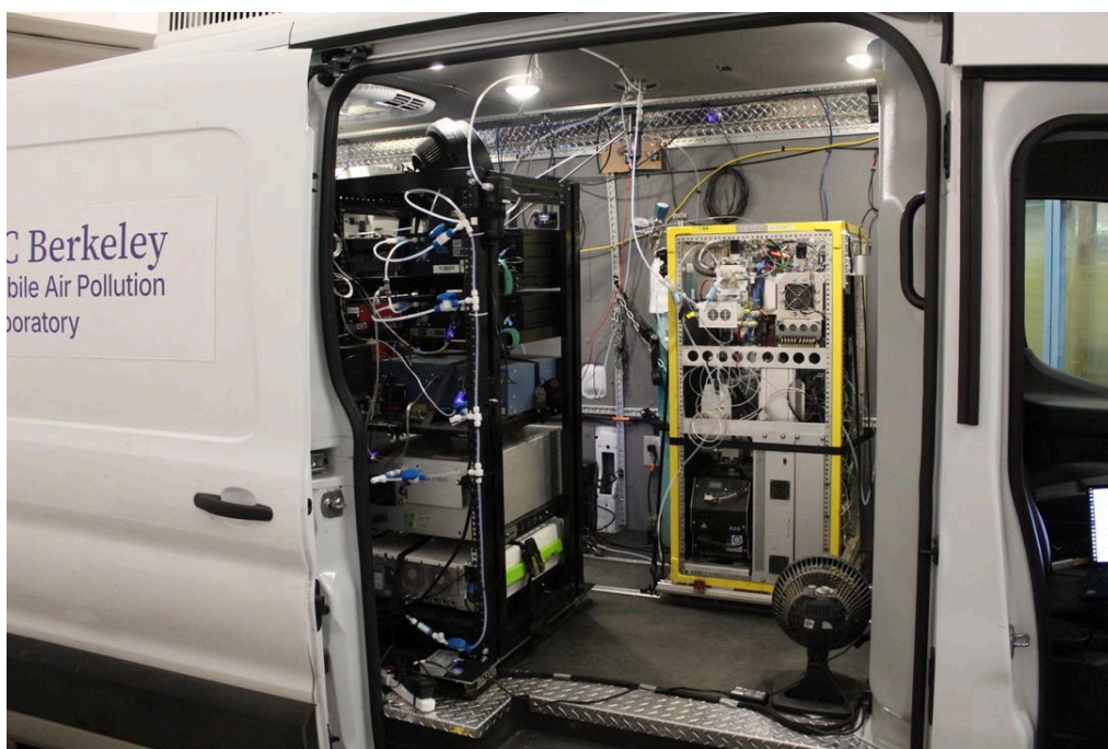
Figure S1: Side on view of the CalMAPLab through the passenger cargo door. On the left is the gas phase rack containing the Aeris CH 4 /C 2 H 6 , Aeris CO/N 2 O, 2BTech O 3 , CAPS NO 2 and EcoPhysics NO x and on the right is the Vocus PTR-ToF-MS in the yellow rack. Sample lines can be seen entering through the roof inlet plates and distributed to the different instruments.
