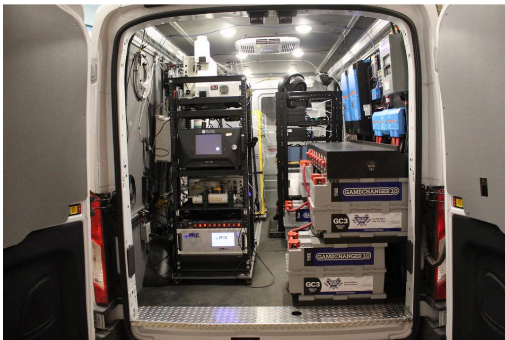
Figure S1: Side on view of the CalMAPLab through the passenger cargo door. On the left is the gas phase rack containing the Aeris CH 4 /C 2 H 6 , Aeris CO/N 2 O, 2BTech O 3 , CAPS NO 2 and EcoPhysics NO x and on the right is the Vocus PTR-ToF-MS in the yellow rack. Sample lines can be seen entering through the roof inlet plates and distributed to the different instruments.
