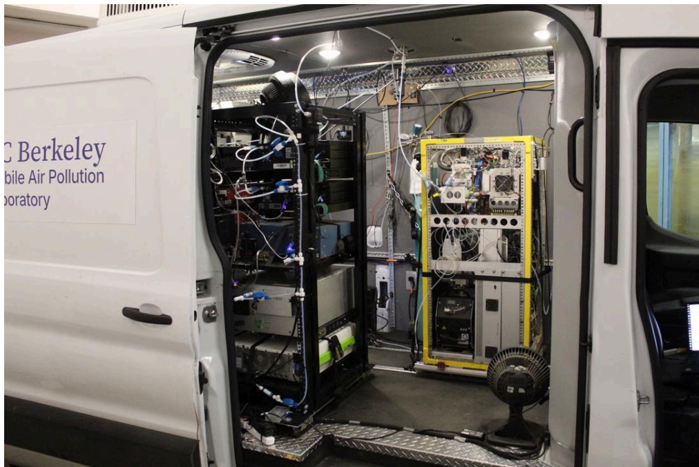
Figure S1: Side on view of the CalMAPLab through the passenger cargo door. On the left is the gas phase rack containing the Aeris CH 4 /C 2 H 6 , Aeris CO/N 2 O, 2BTech O 3 , CAPS NO 2 and EcoPhysics NO x and on the right is the Vocus PTR-ToF-MS in the yellow rack. Sample lines can be seen entering through the roof inlet plates and distributed to the different instruments.
