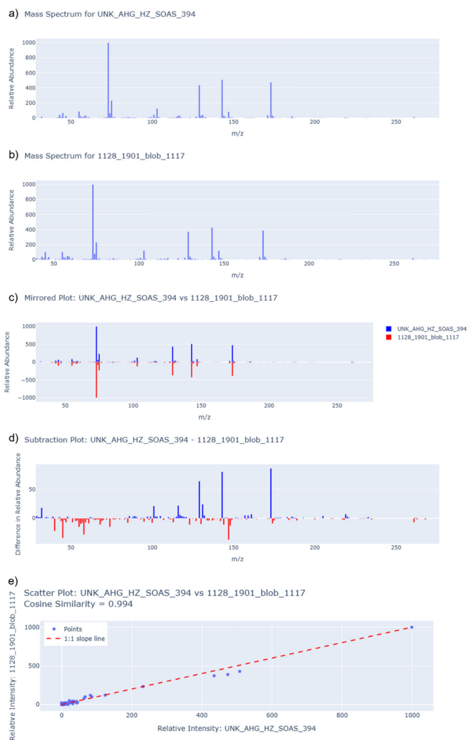
Figure 2: Outputs for MS comparison tool as a) MS for UNK_AHG_SOAS_394 (UID LDY-21509), b) MS for 1128_1901_blob_1117 (UID LDY-22110), c) Mirrored comparison plot for both spectra, d) MS subtraction, and e) Correlation plot of relative intensities with calculated cosine angle similarity between MS.
