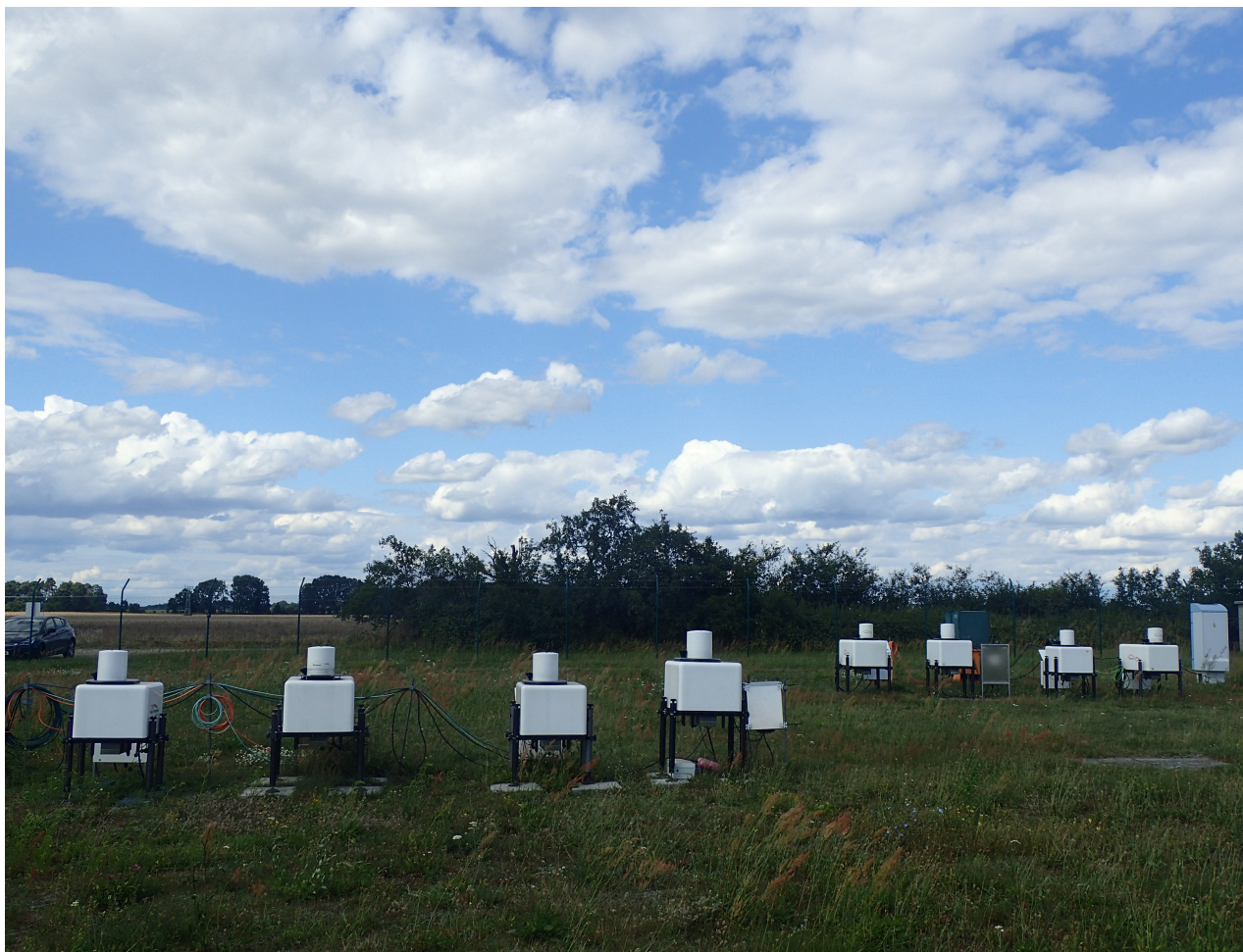
Figure 1. Eight Doppler lidars and a ceilometer operating in the same location at Falkenberg, Germany, during the FESSTVAL Campaign. Photo courtesy of Ronny Leinweber.
