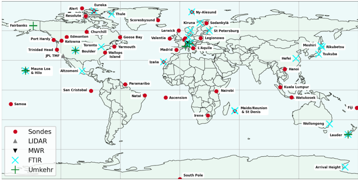
140 Figure 1: Map of all available measurement stations by instrument type: ozonesonde in red, LIDAR in grey, MWR in black, FTIR in cyan and Dobson Umkehr in green.
